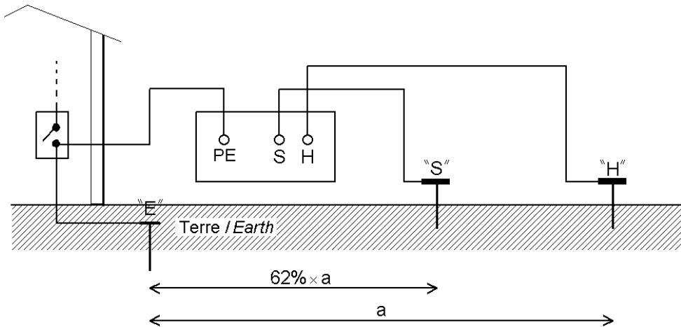
**Remark :** to be sure that rod S is located in a zone that is not influenced by other earth electrodes, move it ( 10% of the distance and repeat the measurement. The result must not change or just from few %.
