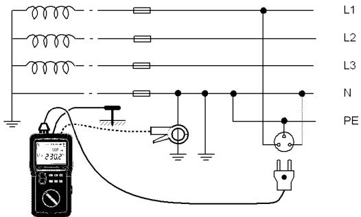
**Note :** without the current probe, what is measured is the global earth of the network, which is not very significant.
