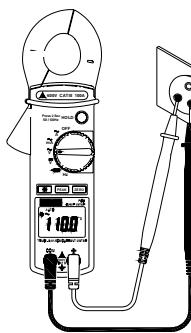
Set the switch to V~ for an AC voltage measurement and to V= for a DC voltage measurement.
