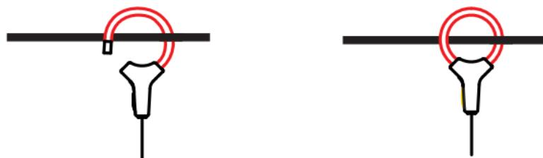
Close the coil. In order to optimize measurement quality, it is best to centre the conductor in the coil and to make the shape of the coil as nearly circular as possible.
