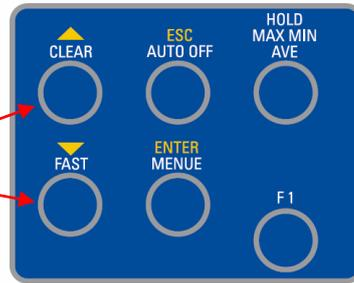
The adjustments of the instruments like the measurement value, calibration of probes, deactivation of channels and so on are resulting from the structure of the menu. You will reach into the main menu by pressing [ENTER/MENUE]. With the up and down keys [↑↓] you can choose your required menu item. Press [ESC] to be back in the measuring mode.
