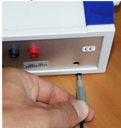
Connect the mains plug with a 230V / 50Hz socket on the rear side. Before switch on the instrument connect the probes on the instrument and take in the calibration number, which is marked on the handle. On the front there are the two probe plugs marked with 1 and 2.
