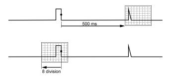
Figure 24. Trigger Delay or Pre-trigger View
