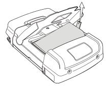
Figure 44. Removing the Battery
