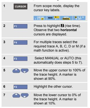
The reading shows the risetime from 10%-90% of the trace amplitude.
