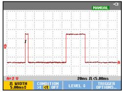
Figure 28. Triggering on Narrow Glitches
