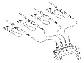
Figure 33. Electronic Connections for Measurements Using Hook Clips and Alligator Clip Grounding
