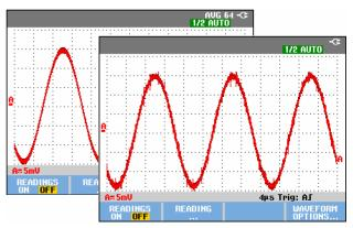
Figure 11. Smoothing a Waveform
