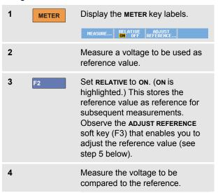
Now the large reading is the actual input value minus the stored reference value. The actual input value is displayed below the large reading (ACTUAL: xxxx), see Figure 10.
