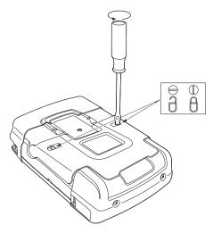
Figure 42. Unlocking the Battery Cover
