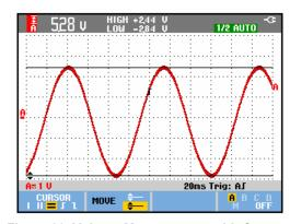
Figure 20. Voltage Measurement with Cursors
