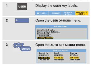
If the frequency range is set to > 15 Hz, the Connect-and-View function responds more quickly. The response is quicker because the test tool is instructed not to analyze low frequency signal components. However, when you measure frequencies lower than 15 Hz, the test tool must be instructed to analyze low frequency components for automatic triggering:
