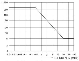
Figure 46. Max. Input Voltage vs. Frequency
