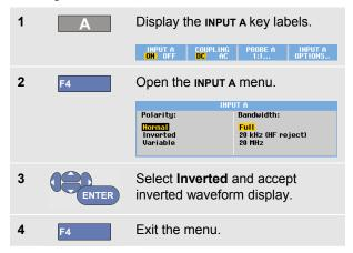
For example, a negative-going waveform is displayed as positive-going waveform which may provide a more meaningful view. An inverted display is identified by an inversed trace identifier ( ) at the right of the waveform, and in the status line below the waveform.
