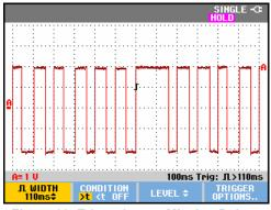
Figure 29. Triggering on Missing Pulses
