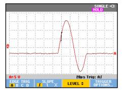
Figure 25. Making a Single Shot Measurement
