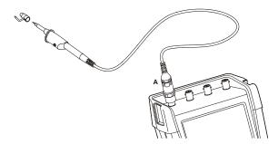
Figure 32. HF Voltage Probe Connection Using Ground Spring
