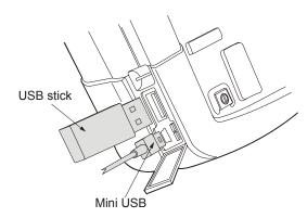
Figure 30. Test Tool USB Connections
