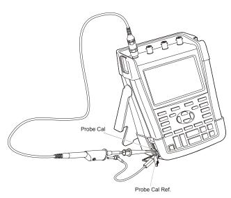
Figure 45. Adjusting Voltage Probes
