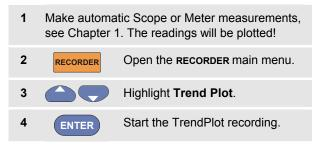
The test tool continuously records the digital readings of the measurements and displays these as a graph. The TrendPlot graph rolls from right to left like a paper chart recorder.
