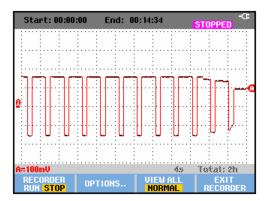
Figure 17. Triggered Single Sweep Recording
