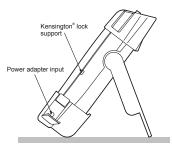
Figure 39. Using the Tilt Stand
