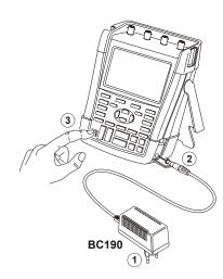
Figure 2. Powering the Test Tool
