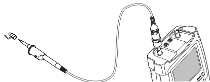
Figure 51. HF Voltage Probe Connection Using Ground Spring
