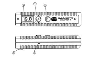
Species selector, setting range 1 - 102 Measuring key ON/OFF (1)4 3 LCD readout (reading in % M.C.) Measuring sensor
