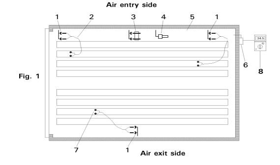
Typical layout of an installation with one each EMC and temperature measuring point and three wood moisture measuring points.
