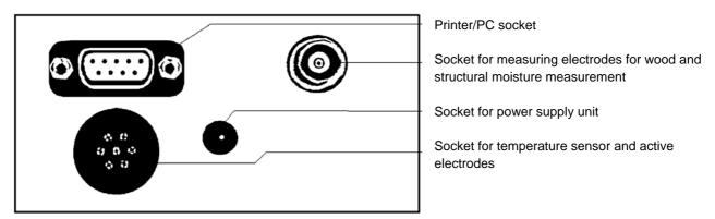
For connection of a printer or a PC, special cables (MK 17 or MK 19) are necessary which are available as optional accessory.
