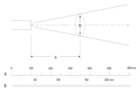
A = Distance between the measuring sensor and the object to be measured
