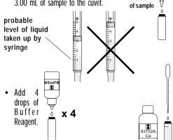
• Use the pipette to fill the cuvet up to the 10 mL mark with the HI 93752A-0 10 mL Ca reagent.
