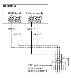
For connecting one HI142 datalogger to the next one, make a cable as explained on the below diagram, by using a 4wire cable and two RJ11 jacks (male connectors):
