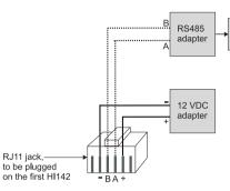
Note: It is recommended to terminate the line of the RS485 network, by plugging on the last HI142 the termination key supplied with the HI504903 supervisor, or connecting a resistor of about  $120\Omega$  as shown here helow
