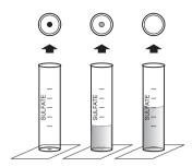
Read the concentration in mg/L (ppm) of Sulfate, in correspondence of the level of the liquid in the test tube.
