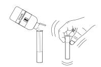
• Remove the cap and add the specific test reagent: Total Chlorine: 1 packet of Free Chlorine: 1 packet of HI 93701-0 Reagent. HI 93711-0 Reagent.
