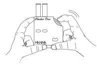
• To measure chlorine in the **0-3.5 mg/L** range, remove the disc, mirror and its holder, if pre-installed. Then install just the disc as shown here.
