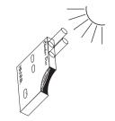
• Keep the checker disc at a distance of 30-40 cm (12-16") from the eyes to match the color. Rotate the disc while looking at the color test windows and stop when you find the color match. Read the value in the result window and divide it by 5 to obtain mg/L (or ppm) of Chlorine.
