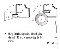
• Insert one of the vials into the left hand opening of the checker disc. This is the blank.
