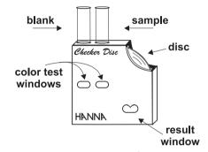
Add to the other glass vial 2 drops of pH Wide Range Indicator. Replace the cap and mix the solution by gently swirling. This is the reacted sample.
