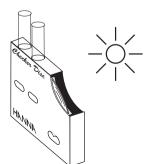
Rotate the disc while looking at the color test windows and stop when you find the color match. Read the value in the result window directly in pH units.
