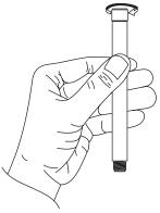
3.) Using dropper provided, add about 2 mL of carbon dioxide internal fill solution HI 4005-40 into outer probe body.
