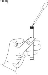
4) Insert and position the inner glass/reference assembly into the outer body so that the anti-rotation key sits in the cut out on the outer probe body.
