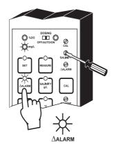
The alarm contacts of **HI 8410** remain closed during normal operation. If the measured conductivity level is not within the tolerance of the set value, the alarm contact will be open.
