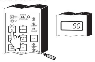
Use a small screwdriver to adjust the COARSE and FINE trimmers until the desired value is displayed in units according with the range selected (the corresponding % DO or mg/L LED is ON).
