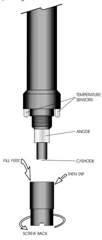
4. With the sensor facing down screw the cap clockwise to the end of the threads. Some electrolyte will overflow.
