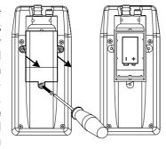
Replacement should take place in a non-hazardous area using a 9V Ni-MH rechargeable battery.
