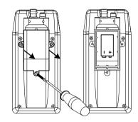
Replacement must only take place in a safe area using an alkaline 9V battery.
