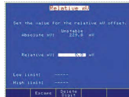
Relative mV calibration allows for a mV offset
