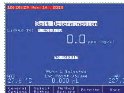
Linked methods allow two methods to run in sequence
