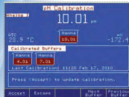
Up to 5 pH calibration points, with automatic buffer recognition
