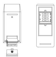
• HI 93501, HI 95502, HI 93503 and HI 935007: the batteries are accessed by separating the front and the back halves of the meter. Unscrew the 4 screws on the back of the meter and carefully replace the three 1.5V AA alkaline batteries located in the battery compartment, while paying attention to their polarity. Reattach the back making sure that the gasket is in place and tighten the 4 screws to ensure a watertight seal.
