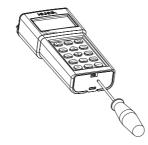
If the battery capacity is less than 20 % the serial communication and the backlight feature are not available.
