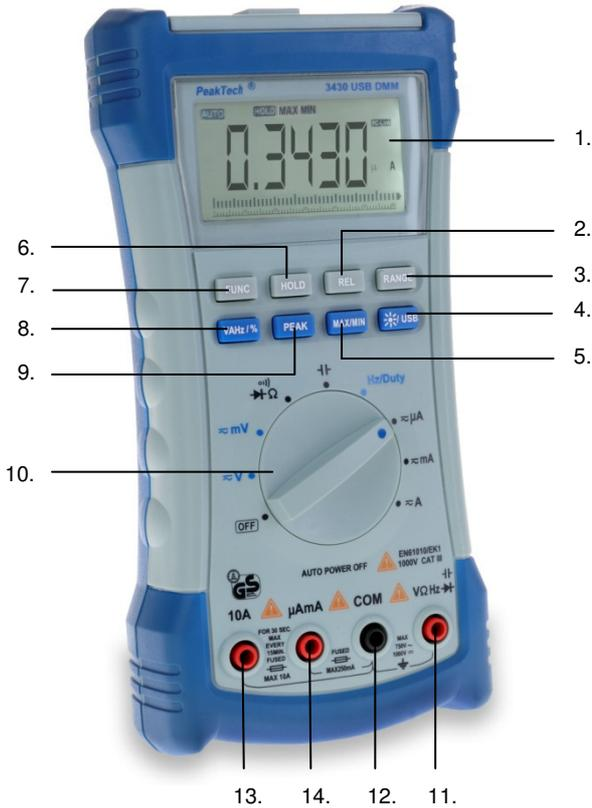
4. For current measurements up to 10A DC, set the function switch to the A position and insert the red test lead into the 10A-jack.
