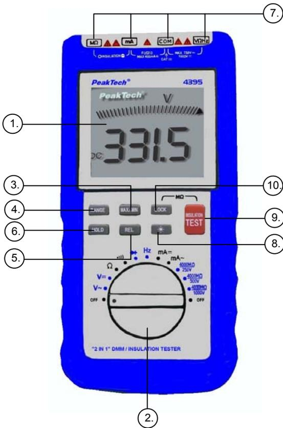
mA For connection of the black test lead during mA-measurements up to 400 mA. Test current input terminal in insulation test, for connection of the black test lead.
