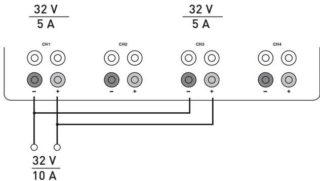
Fig. 7.3: Parallel operation
