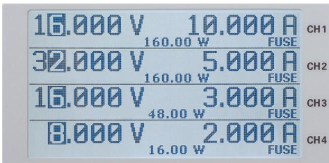
Fig. 5.1: 1 V decimal position of all three channels
