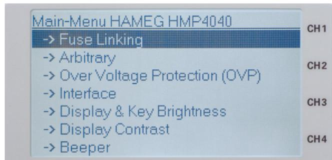
Fig. 5.3: Activated Fuse linking shown in the display
