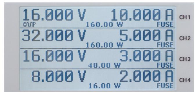
Abb. 5.6: OVP (Over Voltage Protection)
