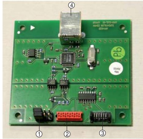
All data and signal lines are electrically isolated from ground.
