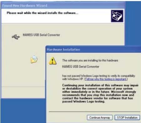
7. Then the "Hardware Installation" window is displayed, showing a warning to continue the installation procedure. As this warning is irrelevant in case of H0870 driver software, click „Continue Anyway“.
