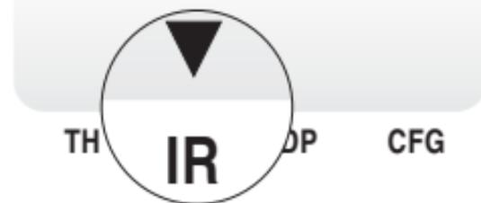
**IR:** The instrument can be used as a **pyrometer** when you select the IR mode. In this mode you can measure the temperature of surfaces without contact. **The instrument**
