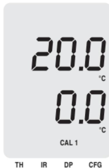
**CAL 1:** The offset for sensor 1 (temperature) is set with CAL 1 (one-point calibration). The offset is shown in the lower display. A maximum  $\pm 10$  °C or  $\pm 10$  °F can be set.
