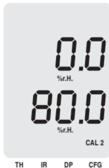
**CAL 2:** The offset for sensor 2 (relative humidity) is set with CAL 2 (one-point calibration). The offset turns the characteristic around the lower calibration point (11 % r.H.). The calibration point must be in the range from 30 % to 95 % r.H. The offset is displayed in the upper display. A maximum  $\pm 10$  % r.H. can be set. **CAL 2 can only be selected in connection with the unit % r.H. and at a prevailing humidity of at least 30 % r.H.**
