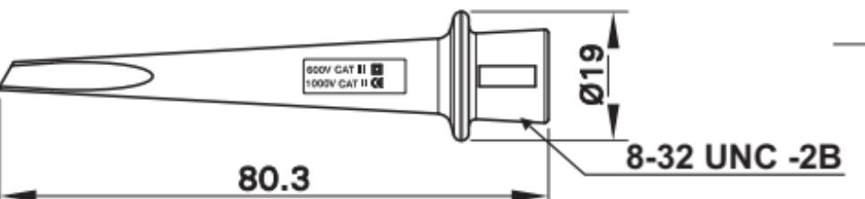
Hook clip with rigid hook. Grasped objects are pressed against the tip of the insulator under spring pressure. Internal thread for attachment to the probes of the test leads XP..../2G.
