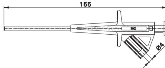
Test clip with flexible shaft and spring wire grabber (stainless steel) for a good contact to pins and wires in inaccessible places. Especially suitable for measuring voltages. The shaft is Silicone insulated and guarantees good heat resistance and flexibility even at low temperatures. Ø 4 mm rigid socket in handle accepting spring-loaded Ø 4 mm plugs with rigid insulating sleeve.
