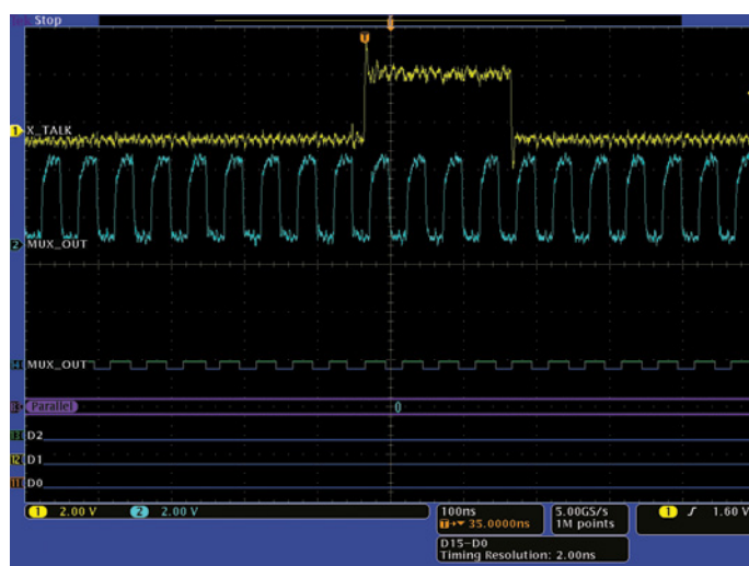
Figure 9. The PCB modification removes the crosstalk.
