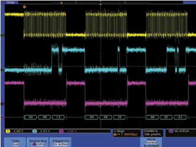
Figure 13. Correct synthesizer configuration messages.
