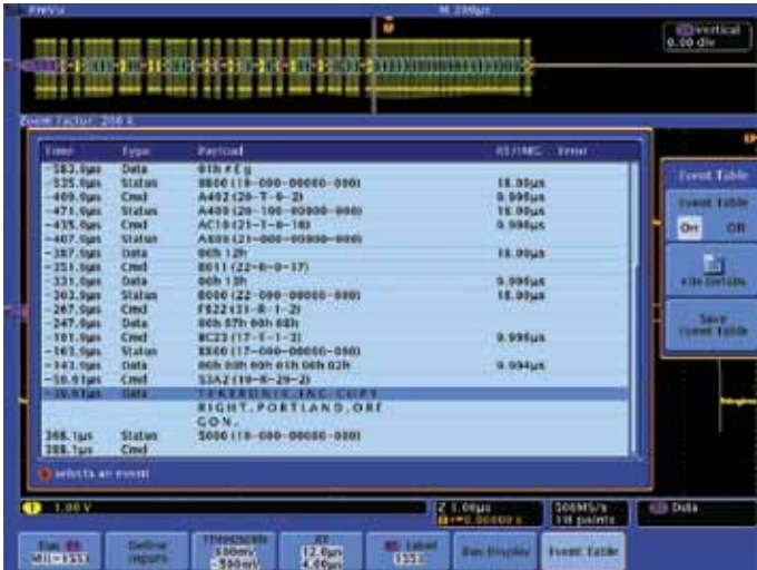
Figure 39. Decoded display of a MIL-STD-1553 bus
