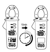
The meter will automatically shut itself off after approximately 10 minutes after power on.
