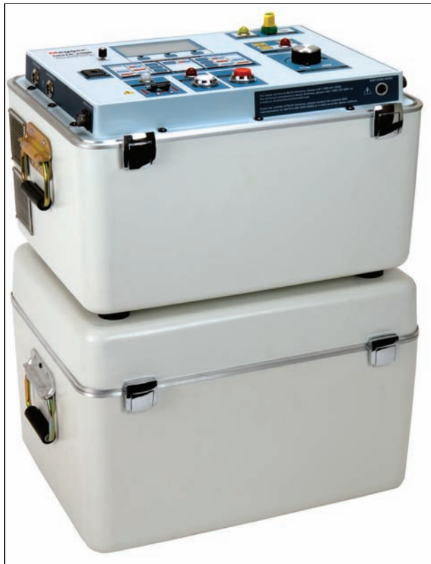
The DELTA2100, available in either 120 or 240 V ac/50 or 60 Hz, includes the control unit (top) and auxiliary module (bottom) containing HV amplifier and LV three-phase TTR circuitry.
