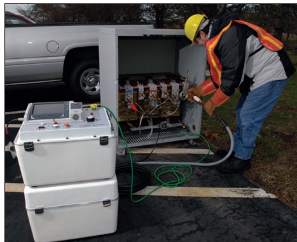
DELTA3000 shown testing a pad mount transformer
