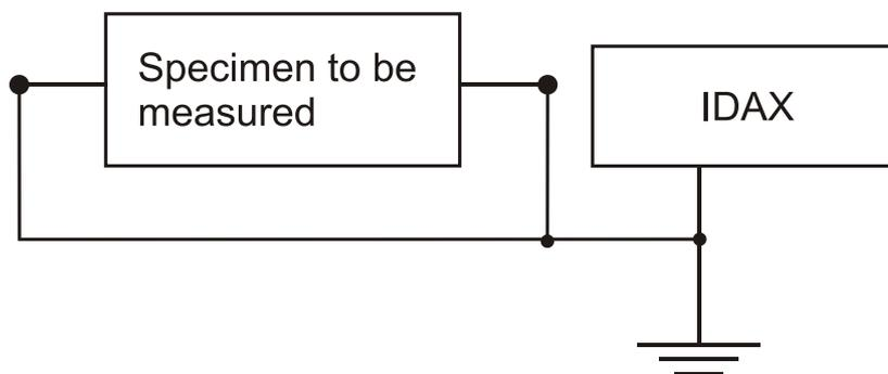
2. In the case of Test Capacitor, keeping the electrodes grounded while connecting IDAX leads is complicated. Therefore, in this particular case with Test Capacitor, it is permitted to remove the ground connections before connecting IDAX.
