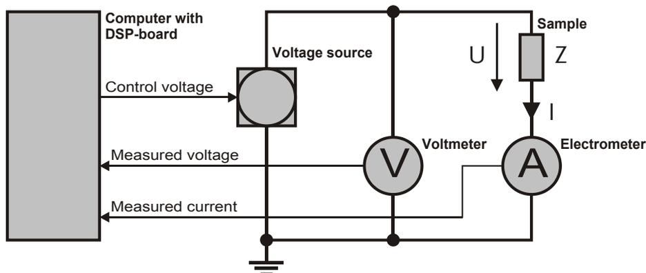
**Fig.1. Measurement of electrical impedance.**
