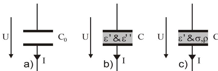
**Material parameter models based on a geometrical capacitance  $C_0$  and material parameters.**
