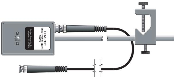
Used to interface the output of the RM-1N Solid State Meter Interface. The RM-1P will operate with both incandescent and infrared optic assemblies. To trigger incandescent source optics, the RM-1P uses a super luminous LED. To trigger infrared (modulated or non-modulated) source optics, the RM-1P uses an infrared sensor and emitter combination. Using the RM-1P with the RM-1N and RM-1H, solid state meters can effectively be interfaced to older test board designs.
