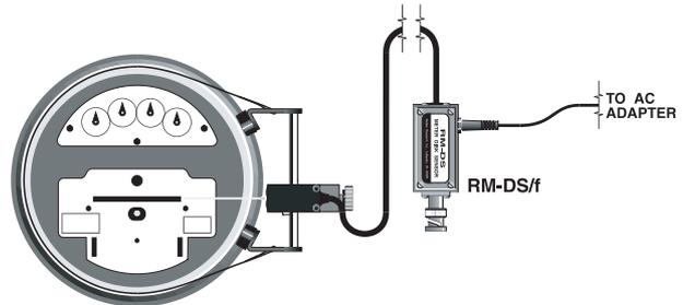
A reflective pickup assembly used to sense the disk rotation of an induction type meter.
