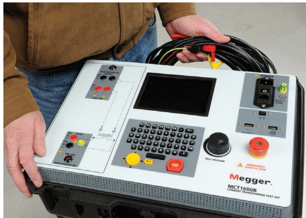
With a manual voltage output control knob, the user is able to perform any test required manually if only a spot check is required.
