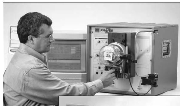
A Universal A-base adapter can easily be installed on a PHAZER Model J120 to facilitate the efficiency of testing both S-base and A-base watt-hour meters.
