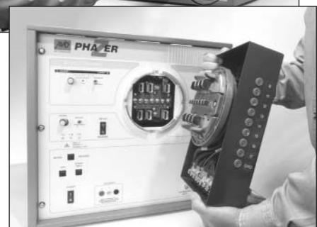
A Universal A-base adapter can easily be installed on a PHAZER Model J120 to facilitate the efficiency of testing both S-base and A-base watt-hour meters.
