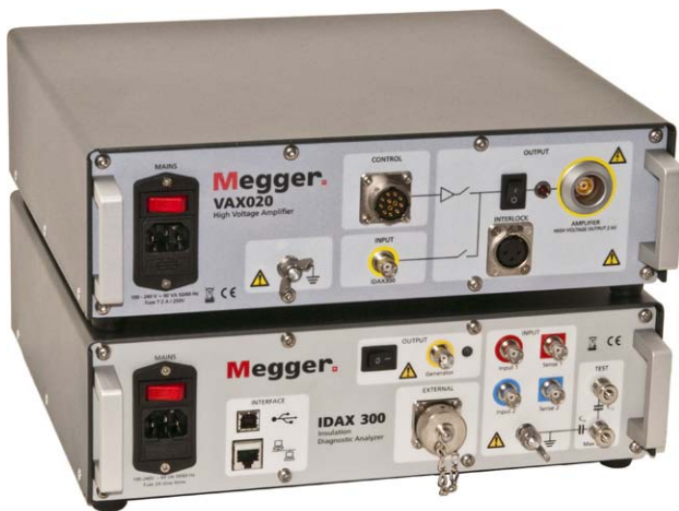
The test system: IDAX-300 and VAX020
