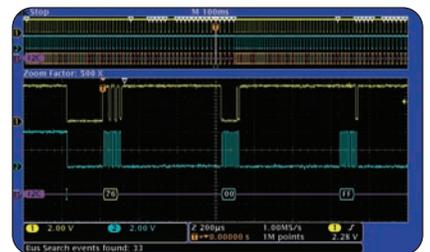
► I<sup>2</sup>C decode showing results from a search for Address value 76. The white triangles indicate each instance of the Address value 76 in the record.
