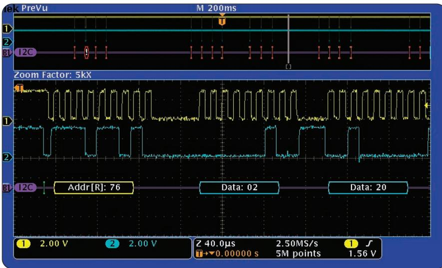
► Triggering on a specific data packet going across an I<sup>2</sup>C bus. The Yellow waveform is clock and the blue waveform is data. A Bus waveform provides decoded packet content including Start, Address, Read/Write, Data and Stop.
