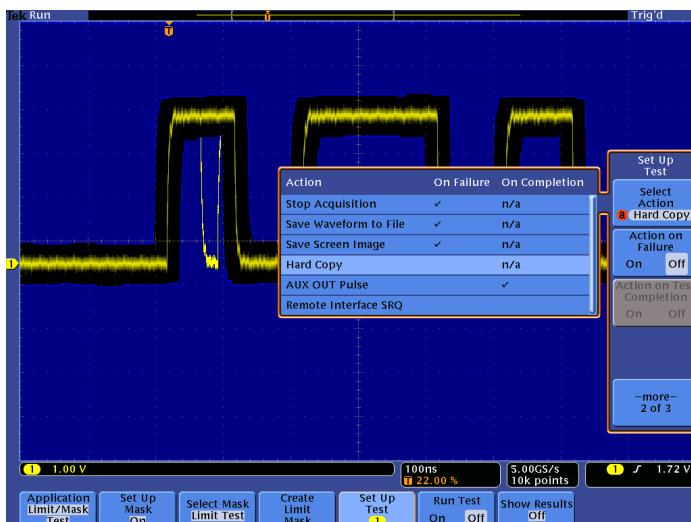
The DPO4LMT Limit and Mask Test Application Module enables multiple actions upon a test failure or the completion of a test, tailoring the test to your specific needs.
