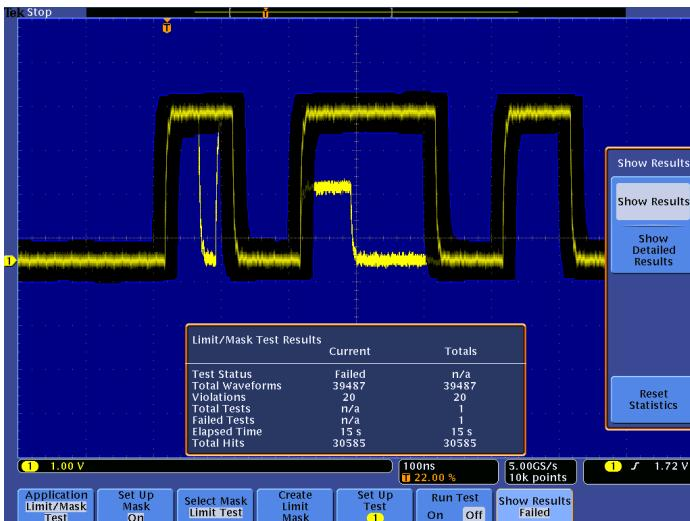
Limit Test finds infrequent glitches and runt signals using a mask created by adding vertical and horizontal tolerances around a golden waveform. Quickly test your signals against a golden waveform and quickly gain insight into anomalous behavior.
