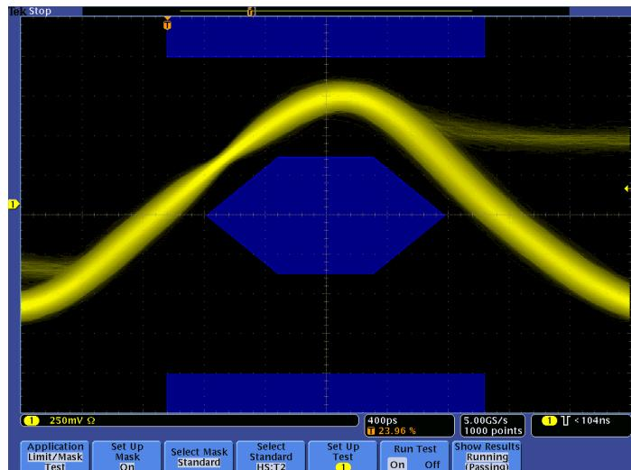
USB 2.0 high-speed standard mask showing results from a mask test. A robust set of telecommunications and computer industry standard masks make testing to standards quick and accurate.
