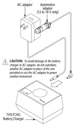
Steady red – charging at full rate Steady green – trickle charging, battery ready Flashing red – battery problem, replace battery
