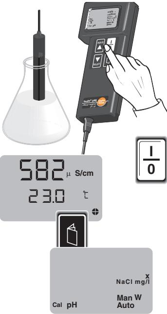
Connect the measuring cell to the instrument.
