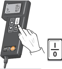
Due to reasons of product engineering, the cell coefficient of the conductivity measuring cell varies. The cell coefficient indicated on the cable of the measuring cell to be used, must be stored in the instrument **before the first measurement**.
