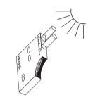
Keep the checker disc at a distance of 30-40 cm (12-16") from the eyes to match the color. Rotate the disc while looking at the color test windows and stop when you find the color match. Read the value in the result window and divide it by 5 to obtain mg/L (or ppm) of Chlorine.
