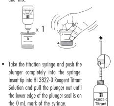
Place the syringe tip into the cap port of the plastic vessel and slowly add the titration solution dropwise, swirling to mix after each drop. Continue adding titration solution until the solution in the plastic vessel changes from colorless to blue.
