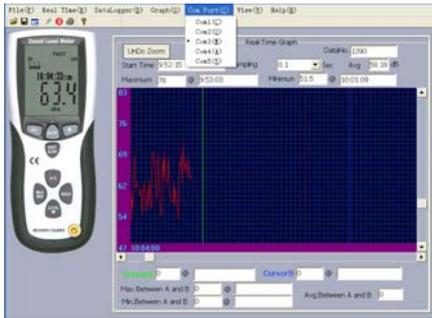
\* Enter the menu “REAL TIME/SETUP” to set the monitoring data(data volume, response, monitoring time)
