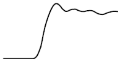
Figure 7: Signal with a long ground lead
