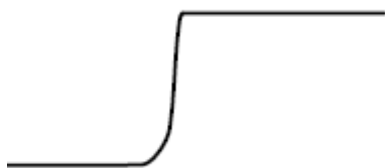
Figure 6: Signal with a short ground lead
