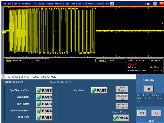
TDSUSB2 compliance test results.
