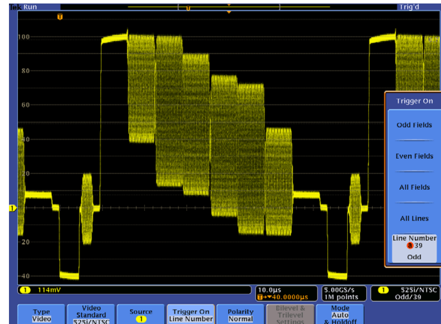
Triggering on line 39 of an NTSC signal
