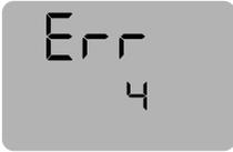
**Slope of the electrode is not within the range -50 mV/pH to -62 mV/pH**
