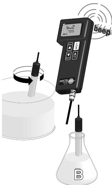
"CAL" flashes during calibration (the calibration lasts for min. 20 sec. and max.10 min.). A signal sounds the end of the calibration procedure. Should the calibration procedure end abruptly after max. 10 minutes, the electrode is probably faulty. Please contact our service department.
