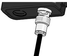
The redox voltage of the solution can be measured by connecting the type 06 mV redox electrode. An NTC probe can be used to measure temperature, although it has no effect on the redox measurement.
