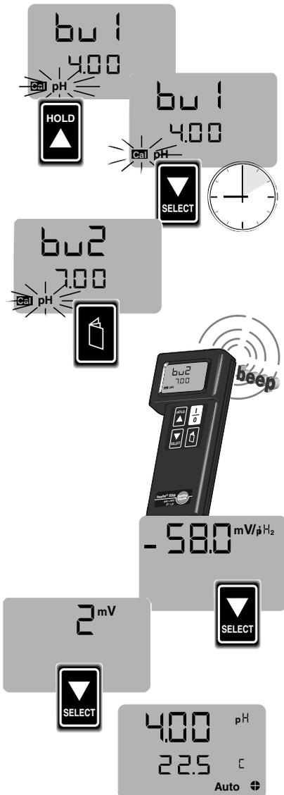
The instrument now asks for the buffer. Select the buffer required with the arrow key (▲) and start the calibration procedure with **SELECT**. The following solutions can be used: pH 1.68 DIN/NBS; 2.00; 4.00; 4.008\* DIN/NBS; 6.865\* DIN/NBS; 7.00; 9.18 DIN/NBS; 10.00
