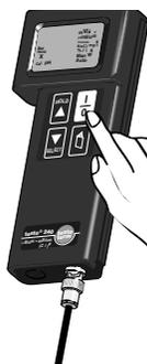
The display indicates the pH value (at first unstable) and temperature.
