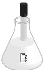
Place the electrode (and the external temp. probe) in the measuring solution.
