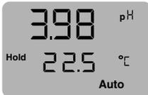
"Hold" appears next to the measured value. The measured value can be held in display as long as necessary, the Auto-off function is deactivated.
