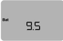
The battery voltage is displayed after the segment test each time the instrument is switched on and can, thus, be checked regularly.
