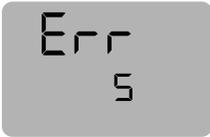
**Zero point of the electrode is not within the range -60 to +60 mV.**
