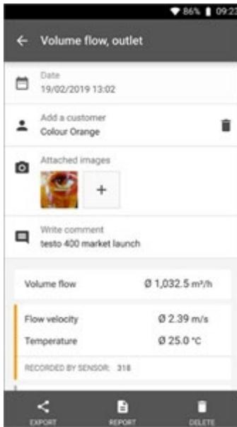
The screenshot shows a measurement detail screen from the testo Smart App. At the top, it displays the measurement type "Volume flow, outlet". Below that is the date "19/02/2019 13:02". There is a section for "Add a customer" with "Colour Orange" listed. Under "Attached images", there is a thumbnail of a photo and a plus sign to add more. A "Write comment" section contains the text "testo 400 market launch". The main measurement data is listed as follows:
